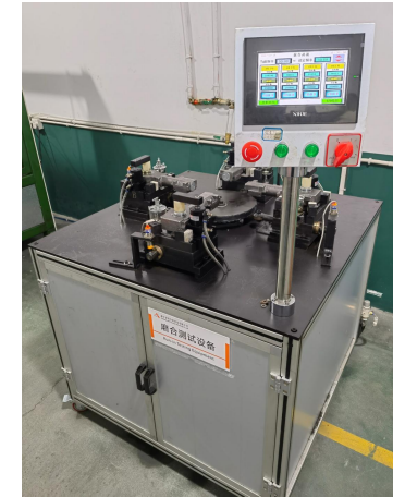
地弹簧&闭门器寿命加速测试机 Floor Spring & Door Closer Accelerated Cycle Testing Instrument
